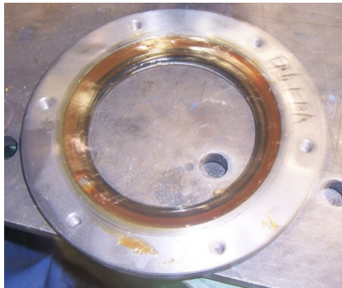
Figure 92 Apply grease to Outer Cover
