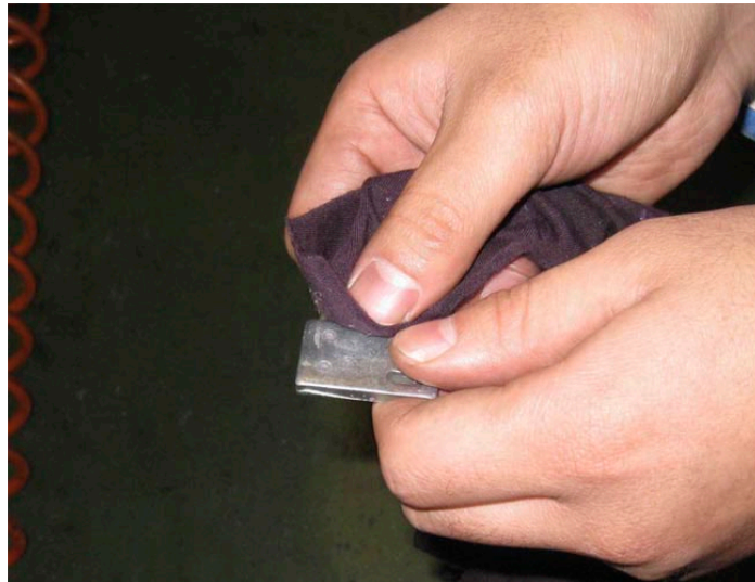
Figure 27 Clean Brake switch bracket
