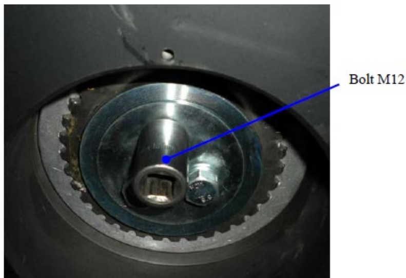
Figure 99 18mm deep well socket on M12 bolt
