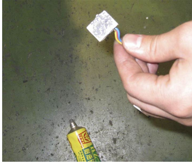
Figure 28 Apply sealant to Brake switch
