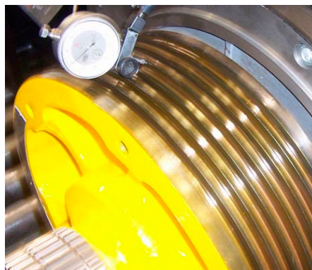
Figure 67 Check groove weave and run out
